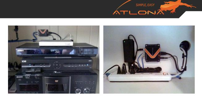
The AT-HD-V40SRS can handle latest HDMI standards including 3D and high resolutions up to 1080p at up to 130ft and 1080i up to 200ft. It is a perfect solution for those who need to extend HDMI signal for a long distance over a single low cost cat5 or cat6 cable.
