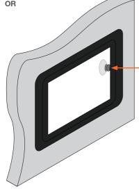
\_Attach the included suction cup to the Velocity Touch Panel and gently pull the panel off the VTP-FMK.
