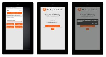
When the installation starts, it will switch to an Android update screen. Once completed it will restart the touch panel. The splash screen will appear, before the loading screen takes over. The update is complete when it returns to the control screen. This process can take up to 5 minutes to complete.
