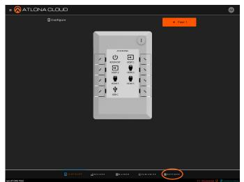
Now that configuration is complete, it must be applied to the unit. Press the Apply button in the top right corner, this will push the configuration to the connected VKP. If the VKP has internet disabled, select Settings in the bottom navigation to open the settings page. Once within settings, select export to download to the local PC for manual upload to the unit. A snapshot can also be saved at this time.
