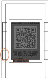
Modes can also be switched by pressing the bottom left hand button from the main screen.
