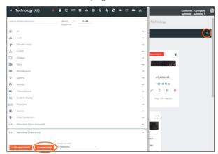
18 Press the scan network button. All Atlona devices found will appear in the unassigned list.
