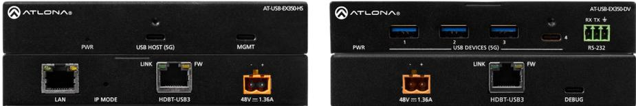
The Atlona **AT-USB-EX350-KIT** is a data only USB 3.2 extender kit. It supports simultaneous extension of 5 Gbps USB 3.2 Gen 1 data and 480 Mbps USB 2.0 data up to 330 feet (100 meters) using a single, cost-effective Category 6A U/FTP cable.
