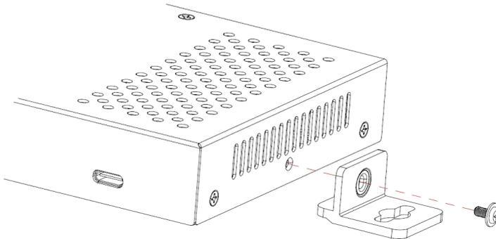
3. Secure the bracket using a small Phillips screwdriver and a screw.
