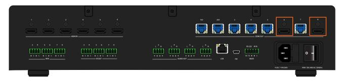
These two HDMI ports are used to mirror (duplicate) an HDBaseT output signal and to either or both HDMI output ports. By default, mirroring is enabled on these two ports. However, mirroring can be disabled. When mirroring is disabled, any of the six HDMI inputs can be routed to these HDMI outputs, transforming this product into an 6 x 8 matrix switcher. The default mirror settings are listed below
