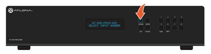
The matrix will power-down and be placed in a low-power state and the **POWER** button will be backlit by a solid red light.
