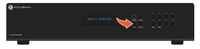
3. Press and release the **INFO** button to display the firmware version.
