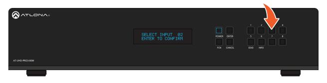
3. Press the **ENTER** button to confirm the selected input. If a different input is desired, press the **CANCEL** button to return to the home screen, then press the button of the desired input.
