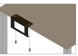
Once secured to the surface, slide the compatible wallplate into the bracket and secure it using the included wallplate screws.
