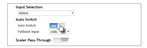
7. Click the **Fallback Input** drop-down list to select the desired mode of operation.
