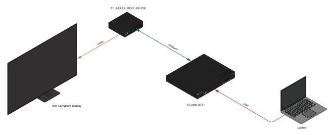
By default, the laptop may transmit HDCP content. However, when connected to a display that does not support HDCP, the laptop must be instructed to send non-HDCP content, in order for the content to be displayed.
