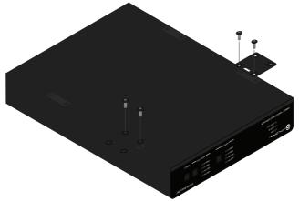
3 Mount the unit using the circular holes, on each mounting plate. Mounting screws are not included.
