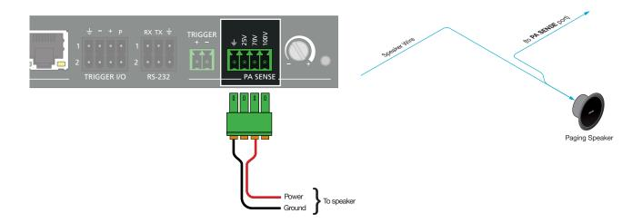
3. Adjust the **PA SENSE** pot to fine-tune the sensitivity.
