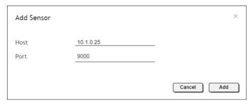
7. Click the **Add** button. If the correct IP address was entered and the AT-OCS-900N is found, information about the sensor will be displayed.
