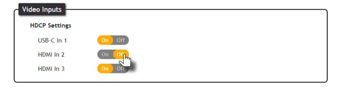
If the display is unable to receive HDCP content, then a "black screen" with no image will be displayed.
