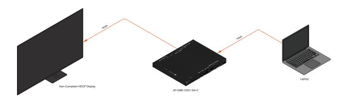
By default, the laptop may transmit HDCP content. However, when connected to a display that does not support HDCP, the laptop must be instructed to send non-HDCP content in order for the content to be displayed.
