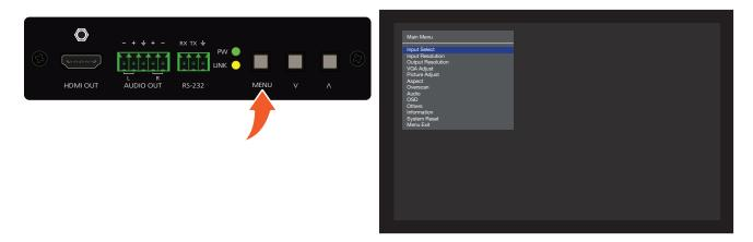
2. Press the **UP/DN** buttons to highlight the various menu options. The currently selected menu item will be highlighted with a blue cursor bar. Press the **UP** button to move the cursor up through the menu system and press the **DN** button to move down.
