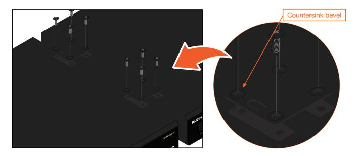
3. Turn the attached units over and install the rack ears (sold separately) to one side of each enclosure using the included screws.
