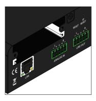
Carefully position the card between the upper and lower rail of each guide, and gently push
