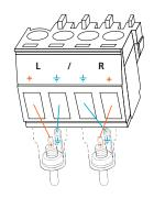
**Note:** Pin outs may vary, please refer to the audio device's manual to ensure a correct connection. **Important!** When terminating cables, please ensure exposed adjacent wires do not touch. This may result in a short that can damage connected devices.
