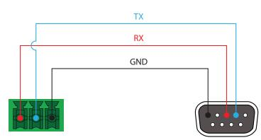
RS-232 is often connected through a DB 9-pin to captive screw connector. The pins will have functions associated with them, some will be unassigned.
