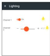
Press and hold the Lighting On button until the Lighting menu opens. This should take 3 to 5 seconds. All lighting controls will appear in the menu. If the control is at minimum it will display a black icon, if on, it will display yellow.
