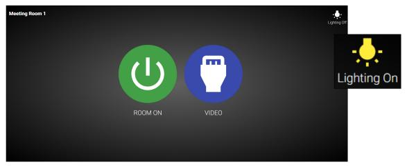
With lighting toggle turned on, simply press the Lighting On button in the top left corner of the screen. This will turn on all channels that were toggle enabled. The icon will turn Yellow when on.
