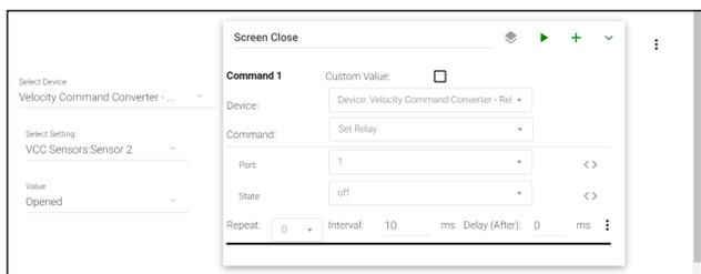
In this example, the sensor being broken will trigger Velocity to set the VCC-Relay port 1 to open. This example will cause the VCC's connected screen to close. It can also be used to trigger the events from the Event Triggers at the same time.
