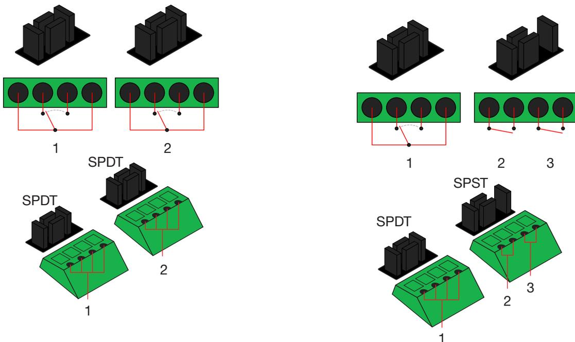
Single Pole, Double-Throw is best used when two circuits are going to one common, such as: switching between two input circuits or selecting two power sources.
