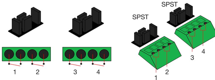
Single Pole, Single-Throw is best used when using a device with a simple open/close (off/on) circuit is being used.
