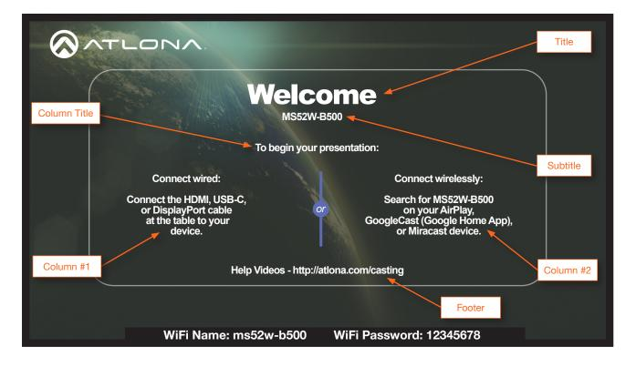
4. Refer to the previous page and make any desired changes to each field. Note that the "tag" {name} is present in the **Subtitle** field, by default. The value of {name} is a system value cannot be changed, as it identifies this specific device: MS52W. However, the {name} tag can be removed from the **Subtitle** field and replaced with other text.
