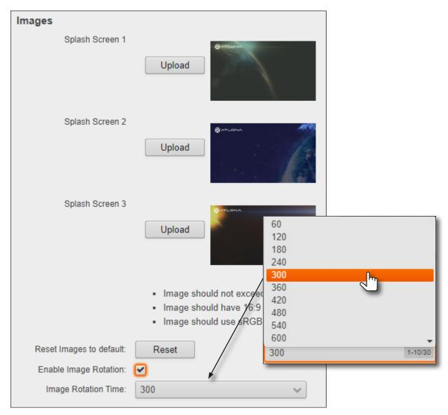
Click the Image Rotation Time drop-down list to select the desired time interval. Range: 1 - 10 minutes. The default image cycling time is 5 minutes (300 seconds). To disable image cycling, uncheck the Enable Image Rotation checkbox.
