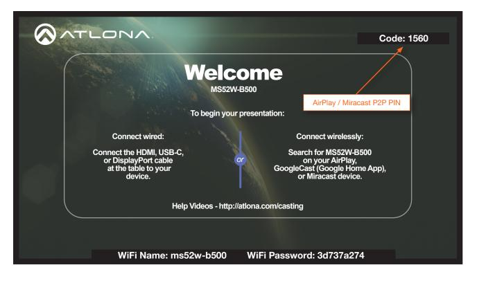
6. Enter the four-digit PIN code in the dialog box on the device and press OK. The PIN code will be displayed only for about 10 seconds. If the PIN code is not entered within the time interval, then the PIN code will be removed from the screen. The example below, shows an AirPlay device prompting for the PIN code. Clicking Cancel in the AirPlay Code dialog box will reconnect the AirPlay device to the AT-OME-MS52W and generate a new PIN code.
