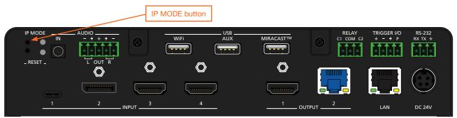
3. Release the **INPUT** button once all the front-panel LED indicators begin to flash. This will cause the unit to reboot which may take up to five minutes. The number of flashes will indicate the currently selected IP mode:
