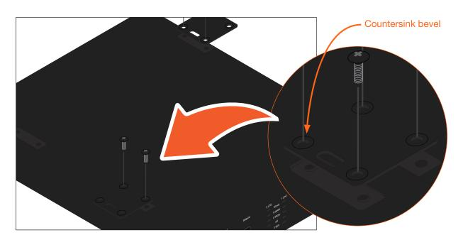
3. Mount the unit using the circular holes, on each mounting plate. If using a drywall surface, a #6 drywall screw is recommended. Mounting screws are not included.
