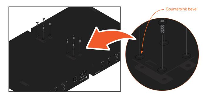
3. Turn the attached units over and install the rack ears (sold separately) to one side of each enclosure using the included screws.
