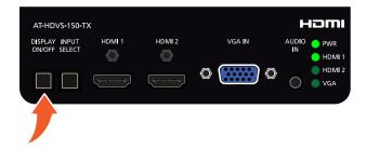
4. While pressing the DISPLAY ON/OFF button, connect the USB cable from the computer to the FW port on the AT-HDVS-150-TX. When the USB cable is connected, the PWR LED indicator will glow solid green.
