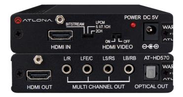
The Atlona HDMI Audio De-embedder and Interface Format Converter includes analog and digital audio outputs, passing up to Dolby TrueHD or DTS-HD Master Audio. Along with multiple audio outputs, the HD570 provides equalized HDMI ports to extend signal up to 15 meters (50 feet).
