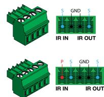
**IR IN** is connected by a ground and signal wire. Use with 3rd party control systems. For easy termination, Atlona recommends using the 2 meter IR cable AT-LC-CS-IR-2M (purchasable through atlona.com).
