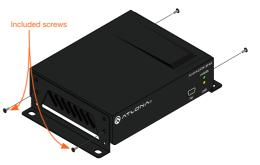
4. Mount the unit using the oval-shaped holes, on each mounting bracket. If using a drywall surface, a #6 drywall screw is recommended.
